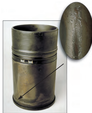
Engine Liner Pitting
