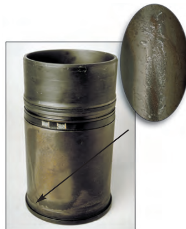
Engine Liner Pitting
